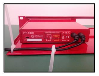
Fish a cable tie through the holes in the rack mount and tie it together. Make sure that the power supply cables are between the holes before fully tightening the cable tie.
