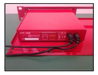
Connect the power cords to the back of the device. Direct the cords to the left as shown in the picture.
