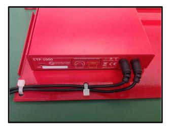
Cut the excess plastic of the cable tie once it has been fully tightened. This allows the power cables to remain secure to the rack mount.
