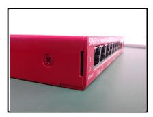
Notice that the Datacom Systems device has a notch on the left side. This notch is used to hold the device until it is screwed in.
