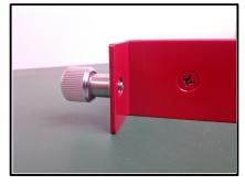
Use the thumbscrew on the other end of the Datacom device to screw it into the rack mount.
