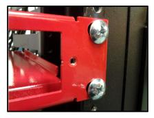
Once the holes on the rack mount and the rack are lined up, use four screws to secure it to the rack.
